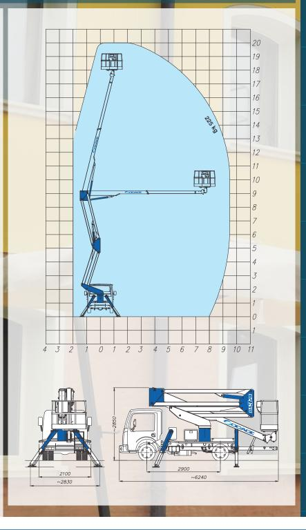
Standard DA Min. Pump Max Max. Max. Weight Cage GVW Series Flow Pressure Heigh Outreach Capacity 1200 kg **DA 320** 3,5 T. 16 l/m 230 bar 20 mt. 9,5 mt. 225 kg
